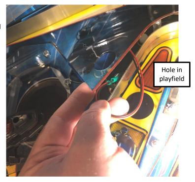
Take the led and place it over the far right exposed stud and push the green rubber over the post, the rubber will keep the led in place and give the metal something to clamp down on and not damage the led light.
